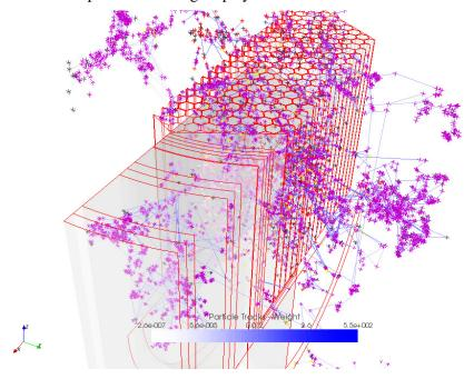
Figure 6. History log colored by event weight on translucent wire frame of reactor with geometry cut away.
