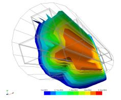
Figure 5: Neutron Dose inside a transport flask
