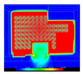
Figure 2. 2D Gamma-Ray dose contours of a dry storage facility.
