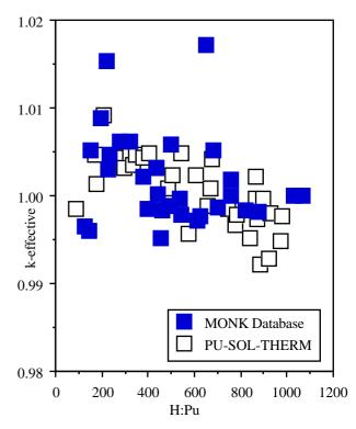
Figure 5 - Calculated k-effective against H:Pu for Plutonium Nitrate Solution Experiments
