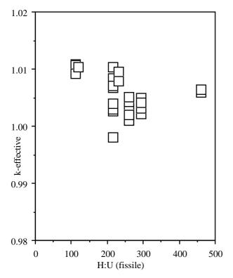
Figure 1 - Calculated k-effective against H:U for Low-enriched Uranium Lattice Experiments
