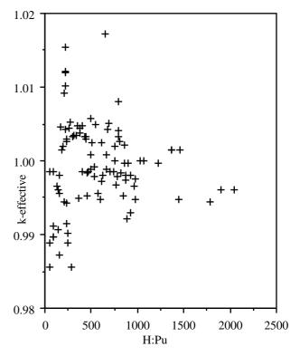
Figure 6 - Calculated k-effective against H:Pu for Nitrate Solution and Mixed Oxide Experiments
