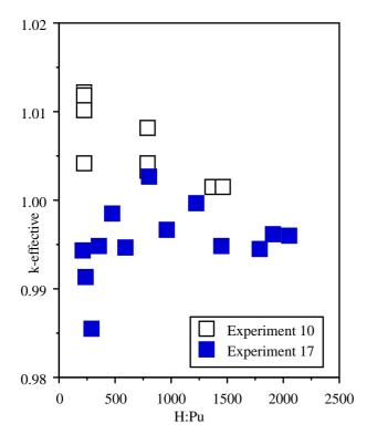
Figure 3 - Calculated k-effective against H:Pu for Mixed Nitrate Solution Experiments
