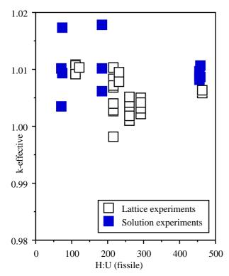
Figure 2 - Calculated k-effective against H:U for Uranium Lattice and Solution Experiments
